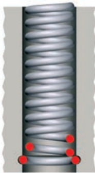
4. Enlarged end coil for mounting in groove
